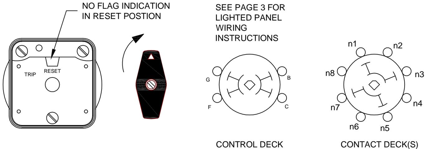
WHEN A PREDETERMINED CONDITION EXISTS, A SIGNAL WILL BE SENT TO S1 WHICH WILL ACTIVATE THE COIL AND CAUSE THE LOR TO "TRIP". THE "B" AND "G" CONTACTS ON THE CONTROL DECK PROVIDE THE CONNECTION TO THE CONTROL CIRCUIT THROUGH S1 WHICH CAN BE A CONTACT OF ANY TYPE I.E. SWITCH, RELAY.... THE LOR CONTACTS IN FIGURE "B" ARE IN THE "TRIPPED" POSITION.
